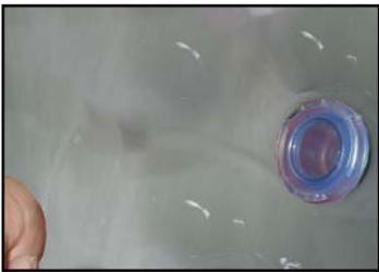
**Step 7.** Re-insert the gasket into clear plastic spout.
