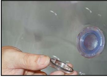
**Step 4.** Pull out the inner plastic filter.
