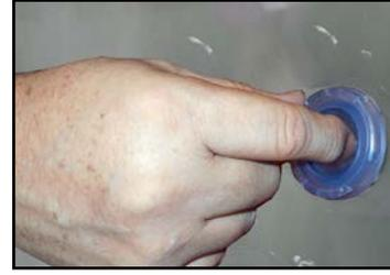
**Step 4.(2)** The plastic filter is shown completely removed from its housing
