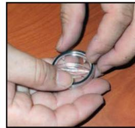
**Step 8.** Place the gasket into the plastic spout and then insert the spout into the jet body.
