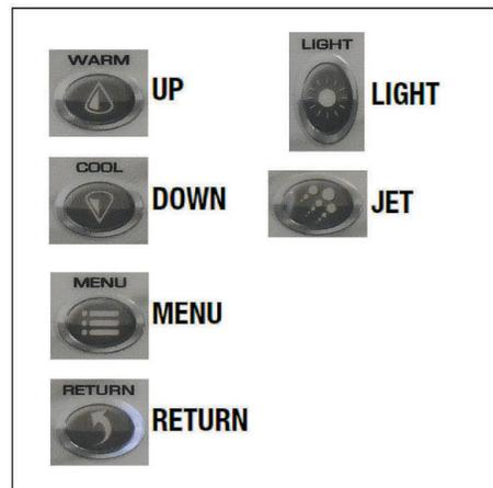
*Default Timeout setting:* Spa **LIGHT** is 60 minutes; **BLOWER** is 15 minutes, **JET** at low speed is 60 minutes; and **JET** at high speed is 15 minutes. User can change these default times in **DEVICE TIMEOUT** setting menu.
