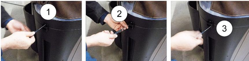
**Step 5** - Keep the cover fastened down at all times when not in use. Locking hardware may be locked with a key (which is provided).
