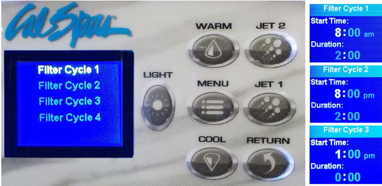
Filter Cycles 1, 2, 3 and 4 can all be adjusted in 15 minute increments. Use the MENU button to move from field to field, use the UP and DOWN arrows to make adjustments and then press RETURN once you're satisfied with your selections for all Cycles. Please note that the system will not allow you to set overlapping or contradictory Cycles.
