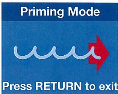
The system will enter the priming mode. **Priming Mode** will display on the control panel. In Priming Mode, all devices such as jets and lights are operable. Jets can be turned on and off to help prime the pump. The system will exit Priming Mode and go to the Main display when the RETURN button is pressed, or after four minutes of inactivity.
