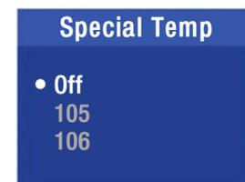
'Special Temp' will heat the spa one time to the selected temperature. The spa will then maintain the previous 'Set Temperature'.
