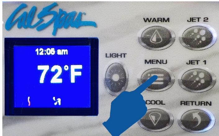
This time select Filter Cycles. (Press the MENU button to access the sub-menus.)
