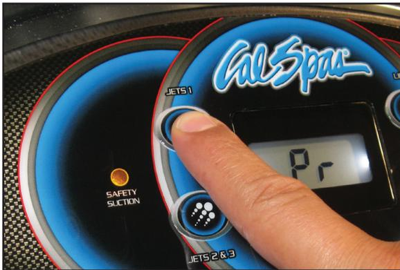
Your spa will perform a self-diagnostic check and go into priming mode. When the control panel displays **PR**, do the following:
