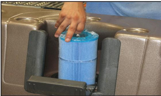
Unscrew the cartridge and remove it.
